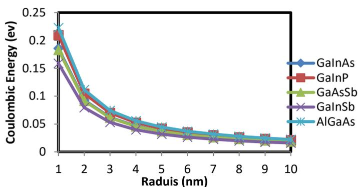
Fig. 2: Variation of Coulombic Energy with radius for some ternary semiconductor quantum dots
