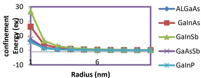
Fig. 1: Variation of confinement energy with radius for some ternary semiconductor quantum dots
