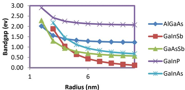
Fig.3: Variation of energy band gap with radius for some ternary semiconductor quantum dots
