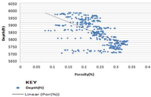
c. Plot showing depth against porosity Geoz 02, Reservoir A
