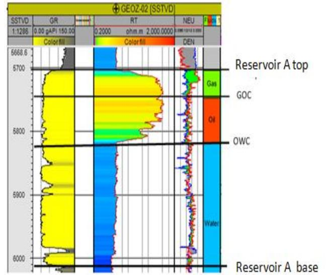
Fig b. Geoz 02 well log for Reservoir A, describing fluid contents and contacts within the reservoir
