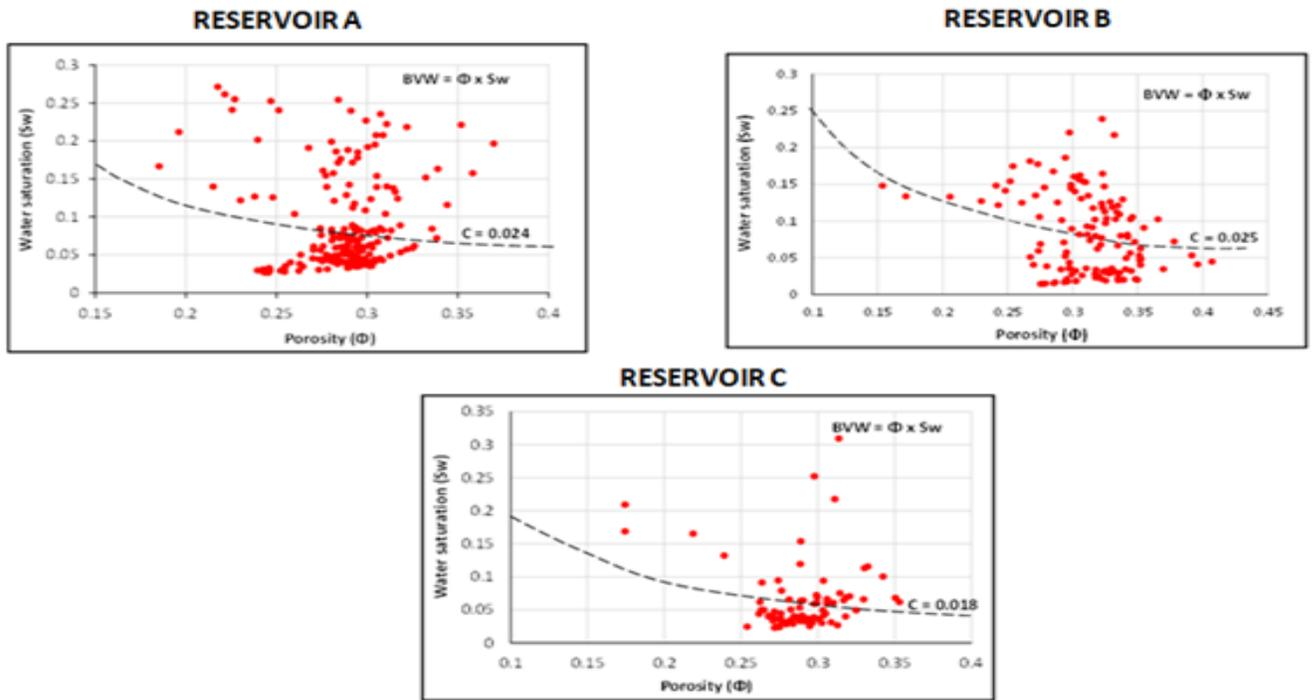
Fig. 5 Bulk volume water (BVW) cross plot for Reservoirs A, B and C in Geoz Field.
