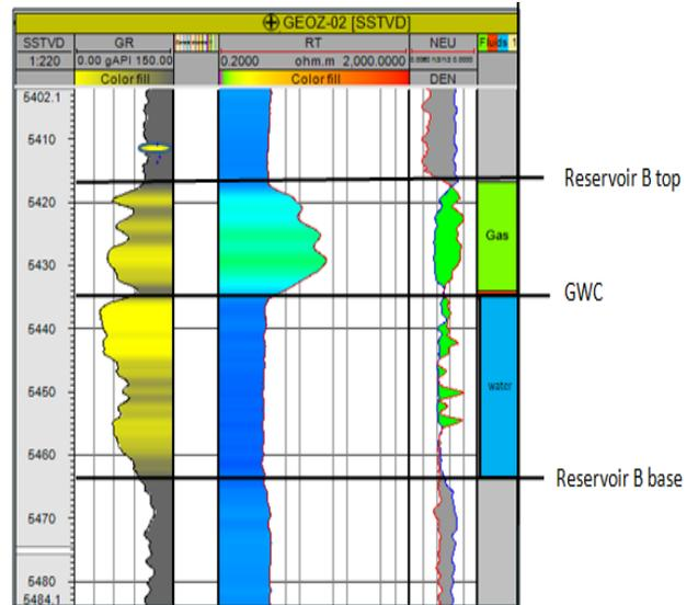
Fig e. Geoz 02 well log for Reservoir B, describing fluid contents and contacts within the reservoir.
