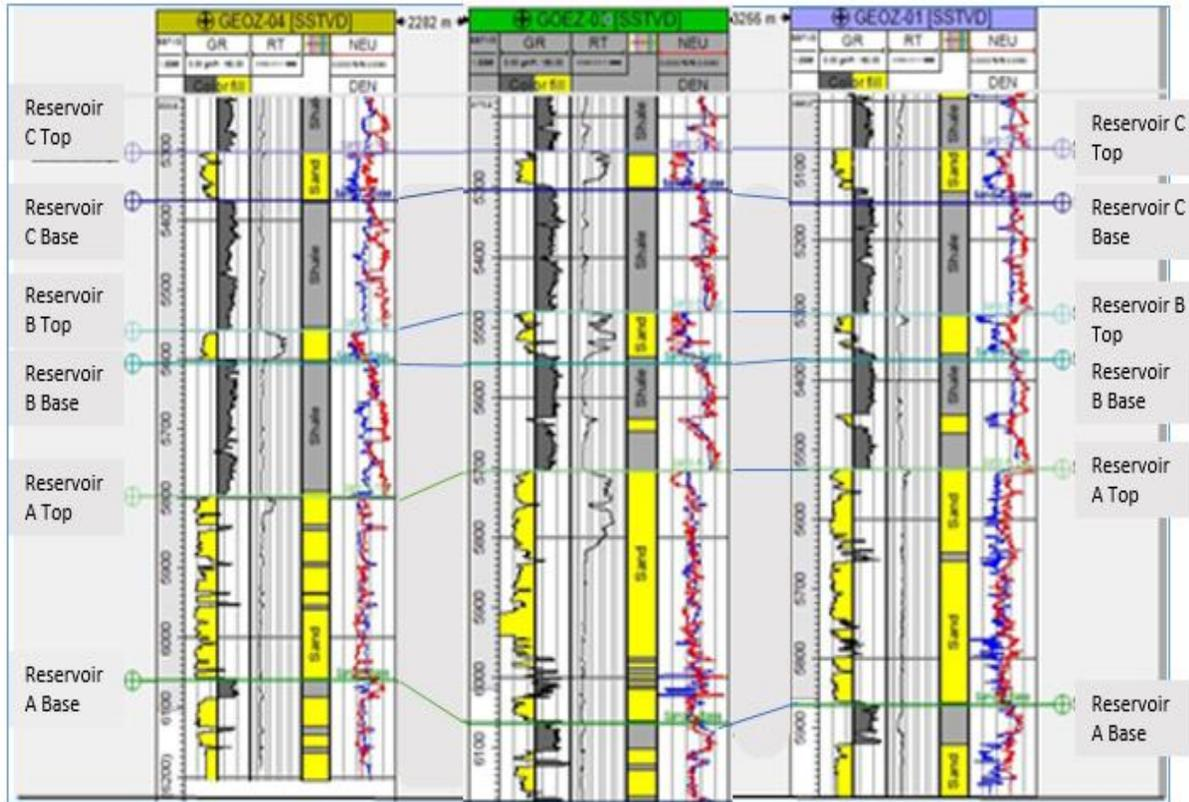
**Fig.7.** Lithostratigraphic correlation of hydrocarbon bearing sands in wells (Geoz 01, 02 and 04) in Niger Delta Basin.
