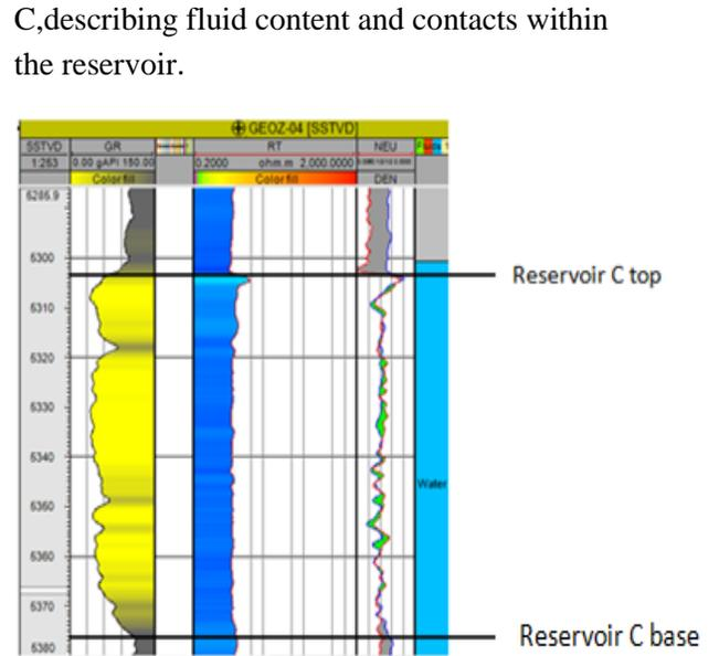
Fig i. Geoz 04 well log for Reservoir C, describing fluid content contacts within the reservoir.
