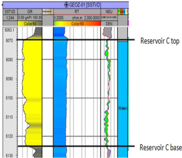
Fig g. Geoz 01 well log for Reservoir C, describing fluid content and contacts within the reservoir.
