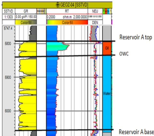
Fig c. Geoz 04 well log for Reservoir A, describing fluid contents and contacts within the reservoir
