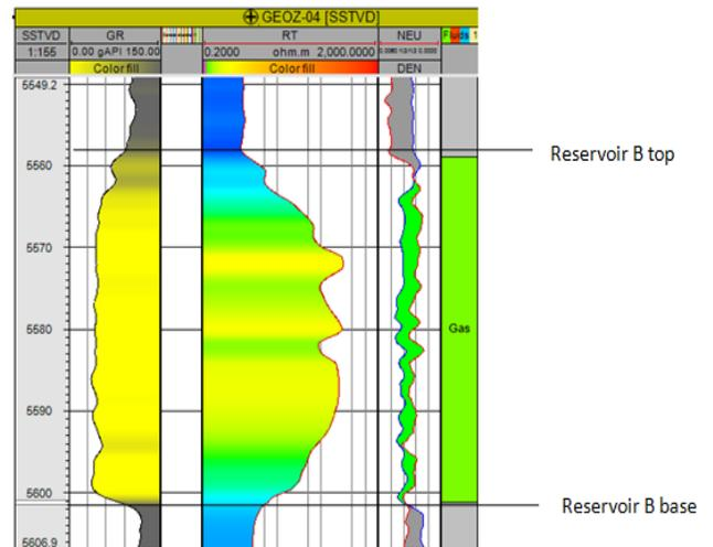
Fig f. Geoz 04 well log for Reservoir B, describing fluid content and contacts within the reservoir
