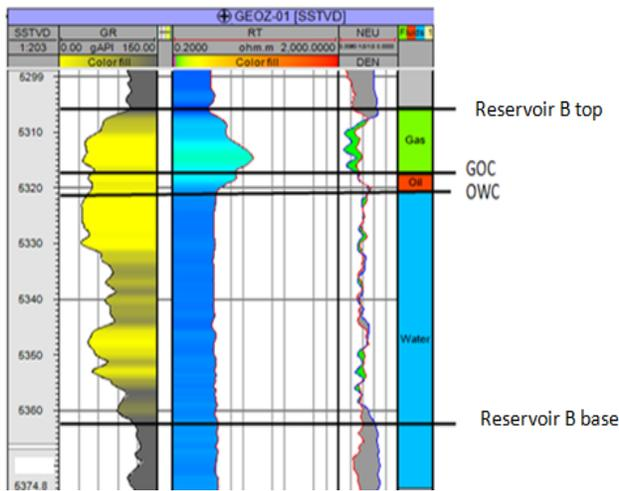
Fig d. Geoz 01 well log for Reservoir B, describing fluid contents and contacts within the reservoir
