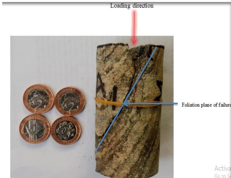
**Figure 7:** Illustration of shear failure in granite gneiss from Okene Southwestern Basement Complex of Nigeria
