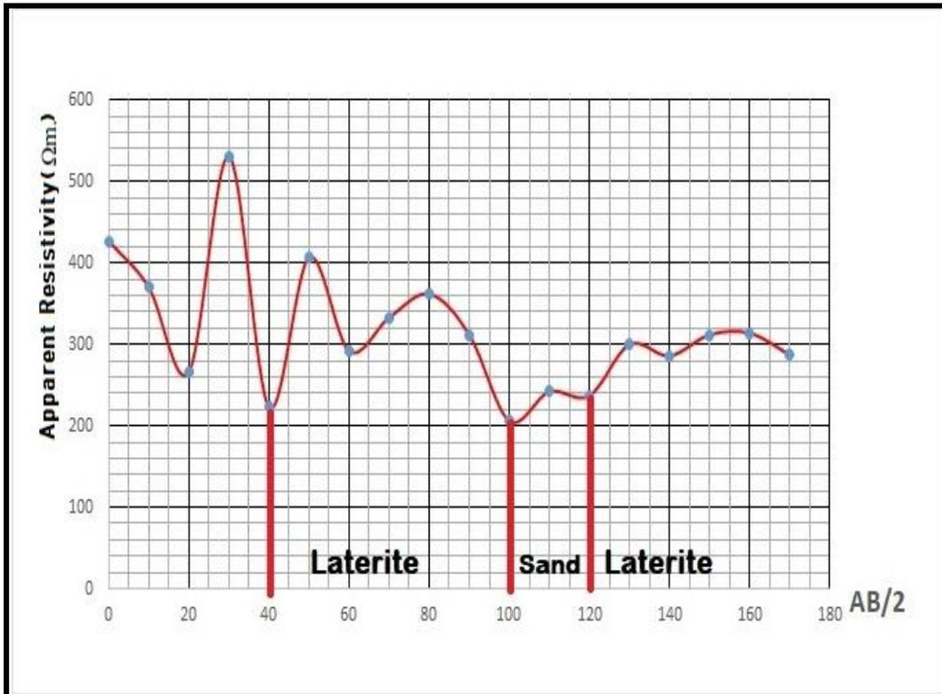
**Figure 6: Wenner profile for Existing Borehole data**
