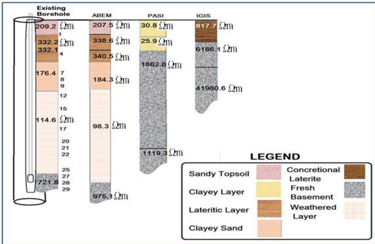
Figure 11: Geo-electric section through the subsurface using the three equipment
