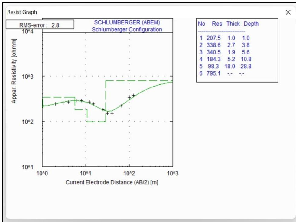
**Figure 3. Iterative curve for ABEM VES data**
