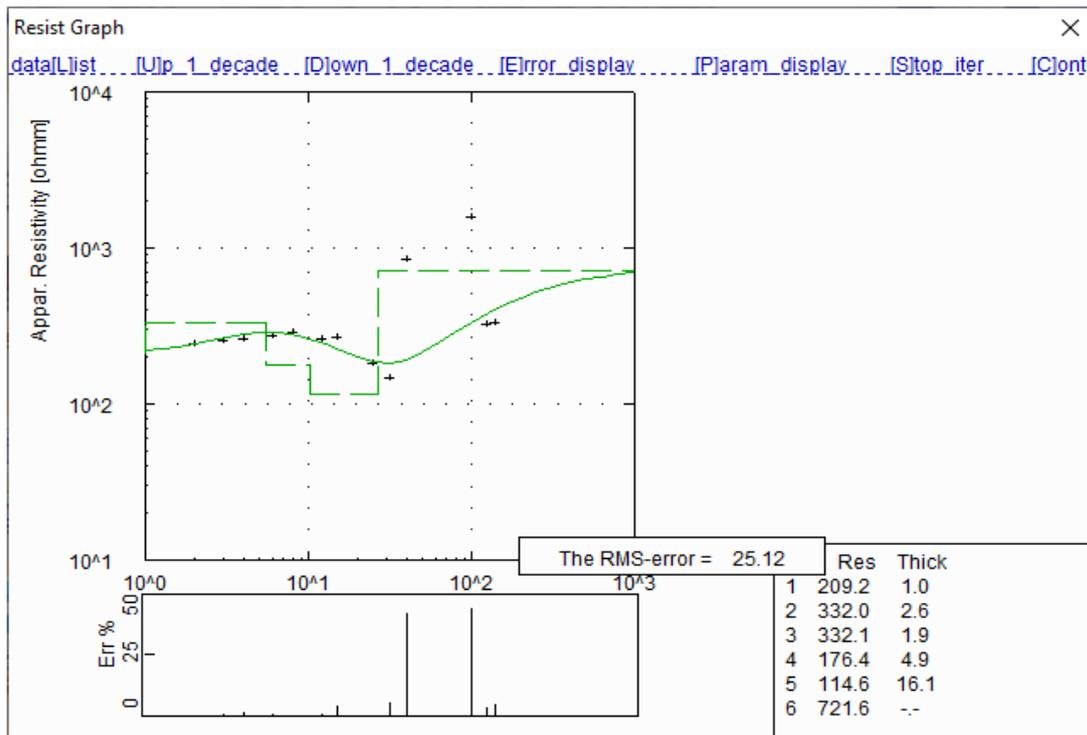
**Figure 2: Iterative Curve for Geosurvey of the existing Borehole**
