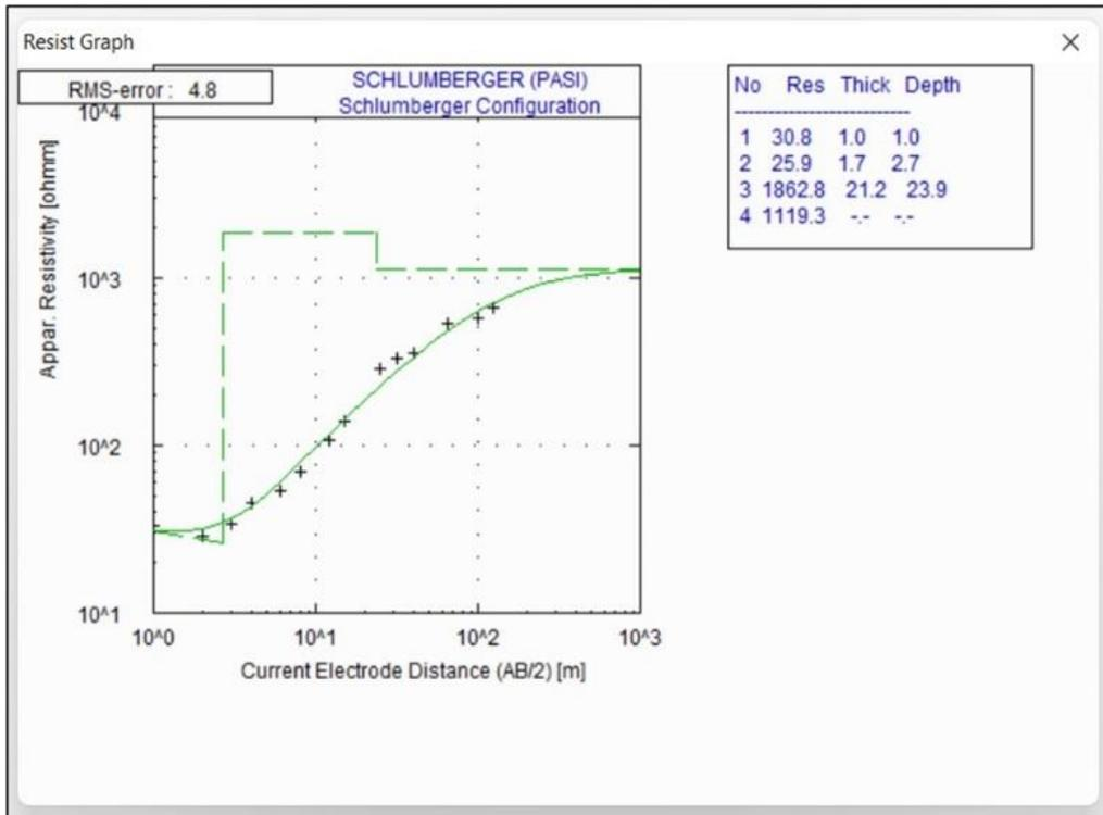
Figure 4: Iterative curve for PASI VES data
