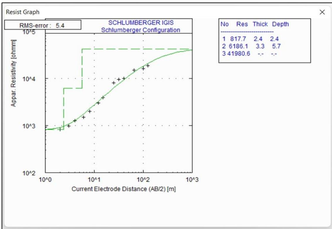
Figure 5: Iterative curve for IGIS VES data
