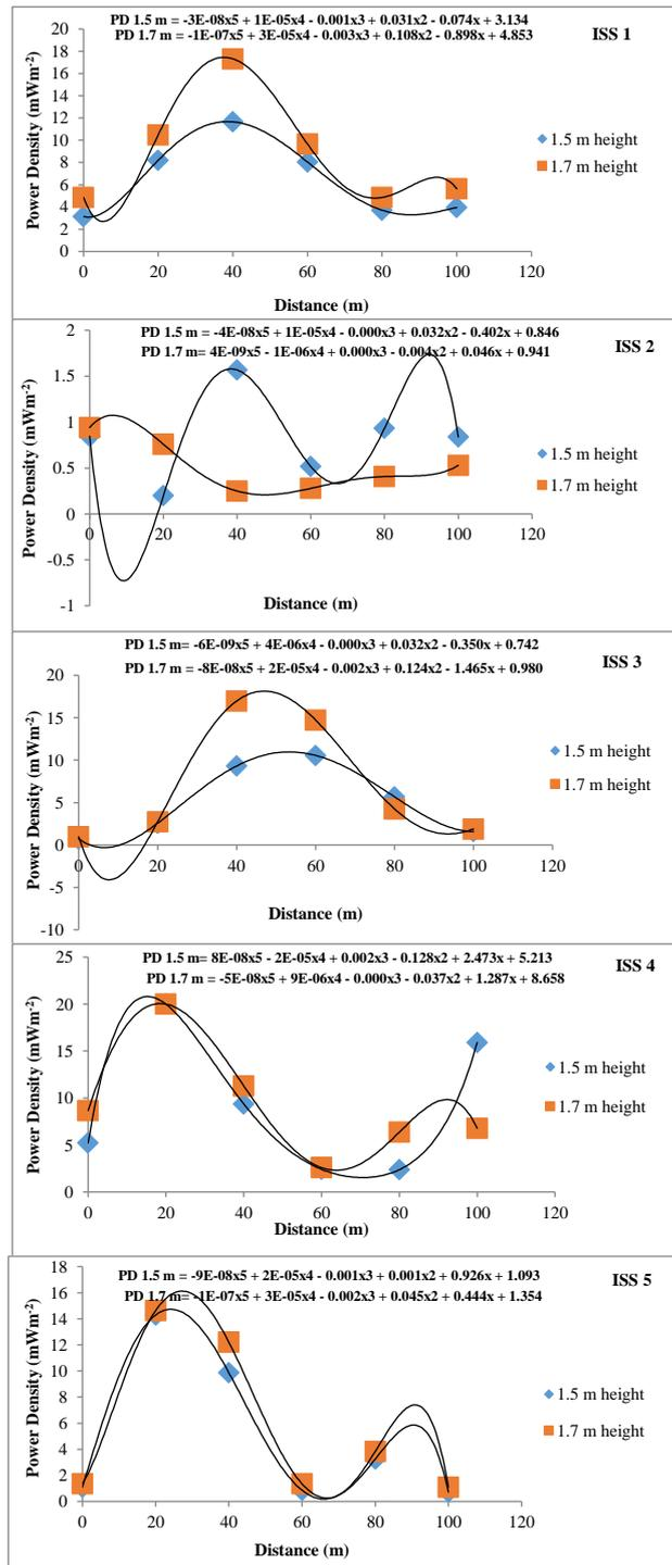
Figure 11: Variation of BTS power density with distance in Isoko South
