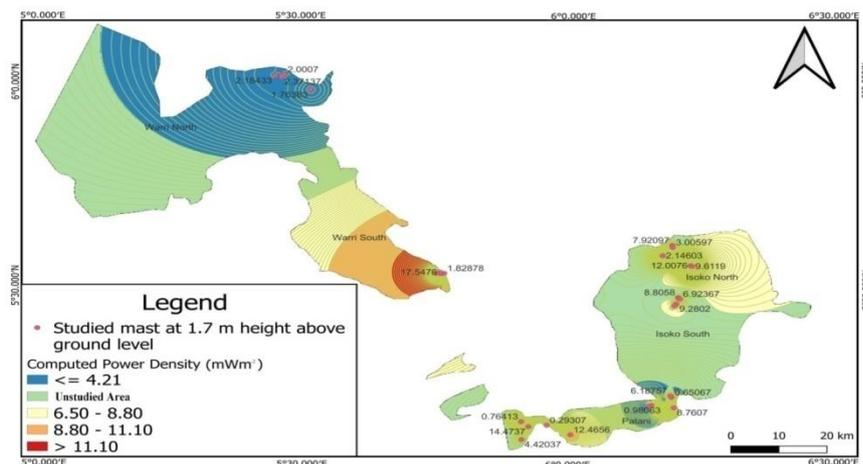
Figure 5: At a height of 1.7 meters, the maximum and minimum RF radiation power density of selected BTSs are distributed on a contour map.
