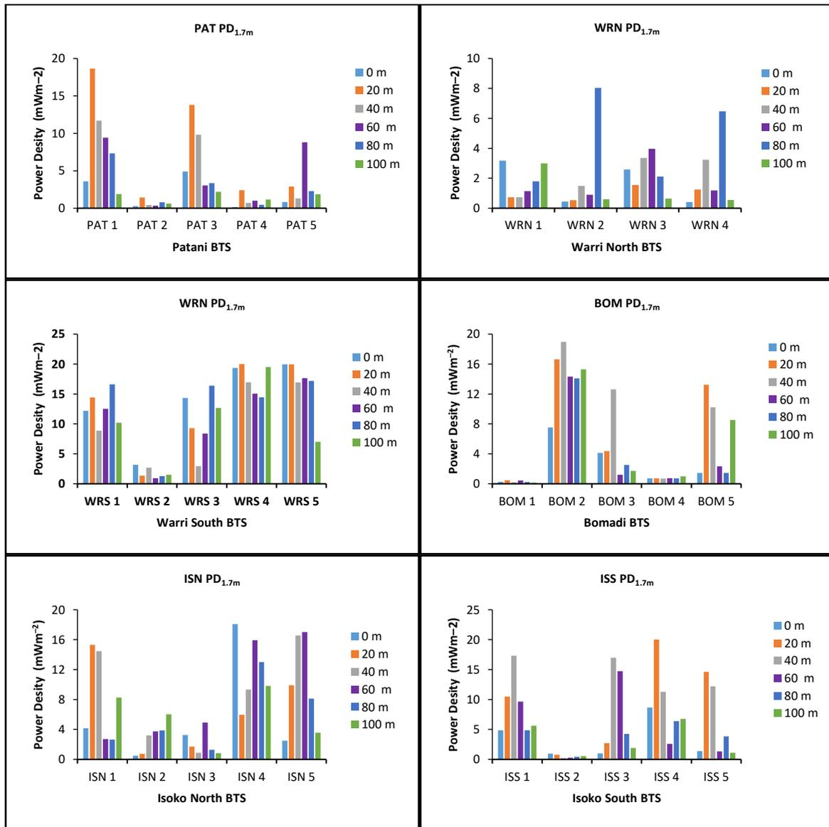
Figure 3: Measured Power density levels of BTS at a height of 1.7 m
