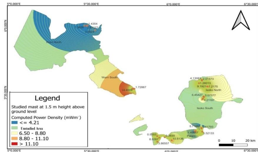
Figure 4: At a height of 1.5 meters, the maximum and minimum RF radiation power density of selected BTSs are distributed on a contour map.
