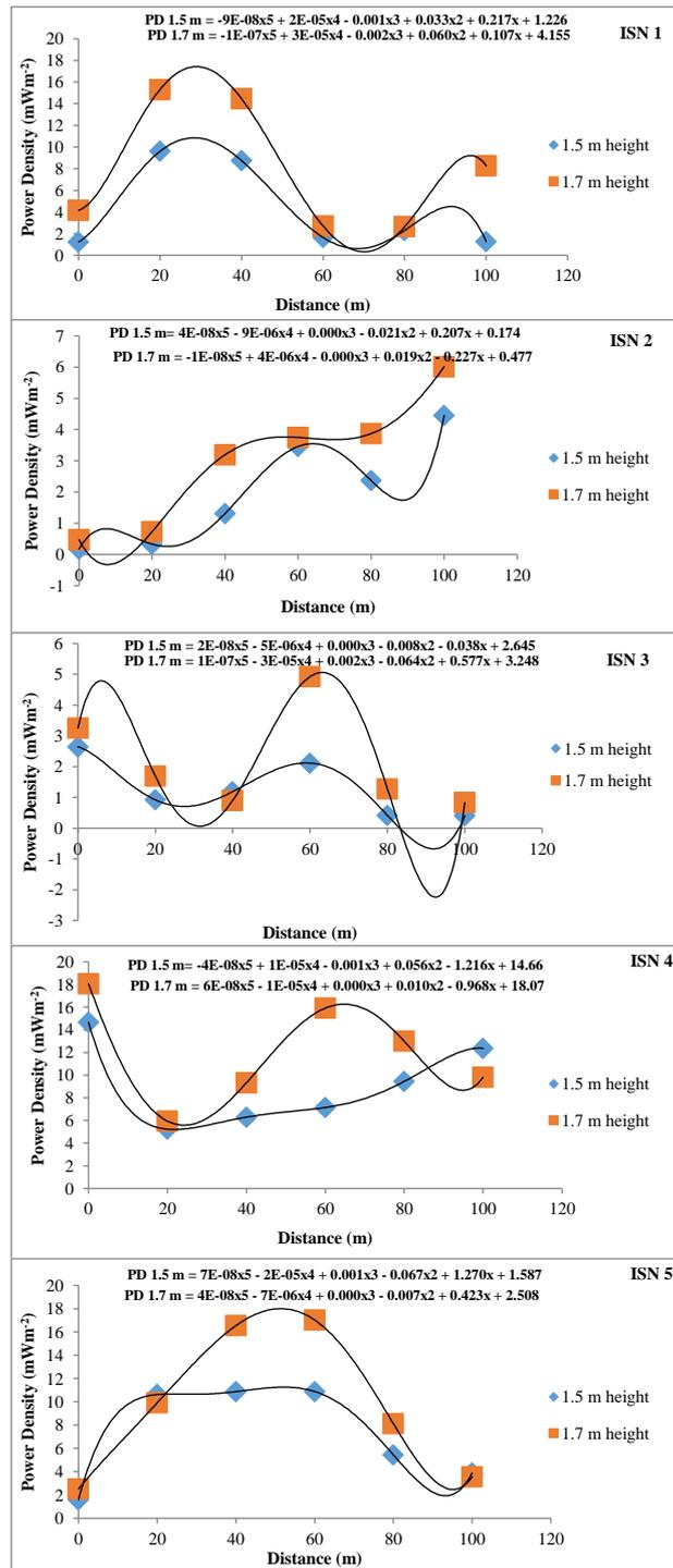
Figure 10: Variation of BTS power density with distance in Isoko North
